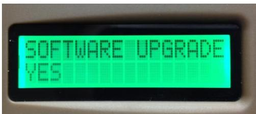
Press the ENTER button once to initiate the software upgrade process. The screen will display UPGRADING for approximately 30 seconds. During this period, do not turn the camera off, or eject the battery tray.
