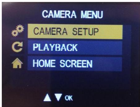
Using the UP or DOWN buttons, scroll through the camera setup options until you reach the option named SOFTWARE UPGRADE , and press the ENTER button.
